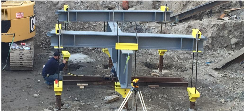
**ONLY SIX TENTHS OF AN INCH NET SETTLEMENT AFTER 24 HOUR LOAD TEST AT FULL LOAD OF 200 TONS!**
